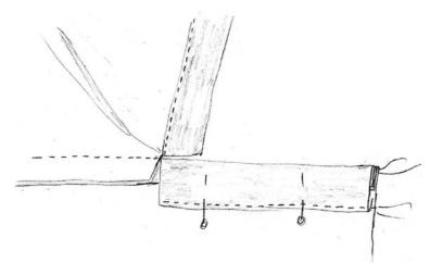
Perform the side seam as a flat felled seam. Trim back seam allowance of the front trouser, fold over the seam allowance of the back trouser and stitch down. Line up button stays
