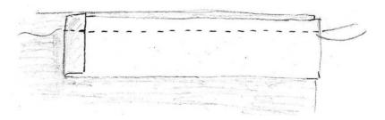
Close side seams respecting marks. Fold in seam allowance of buttonhole facing, fold over the edge and stitch down.
